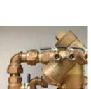
These devices prevent the backflow or "backsiphonage" of non-potable water into the public water supply. Backflow prevention devices operate automatically and come in two different types\*, but both feature a valve that allows water to pass in only one direction.
